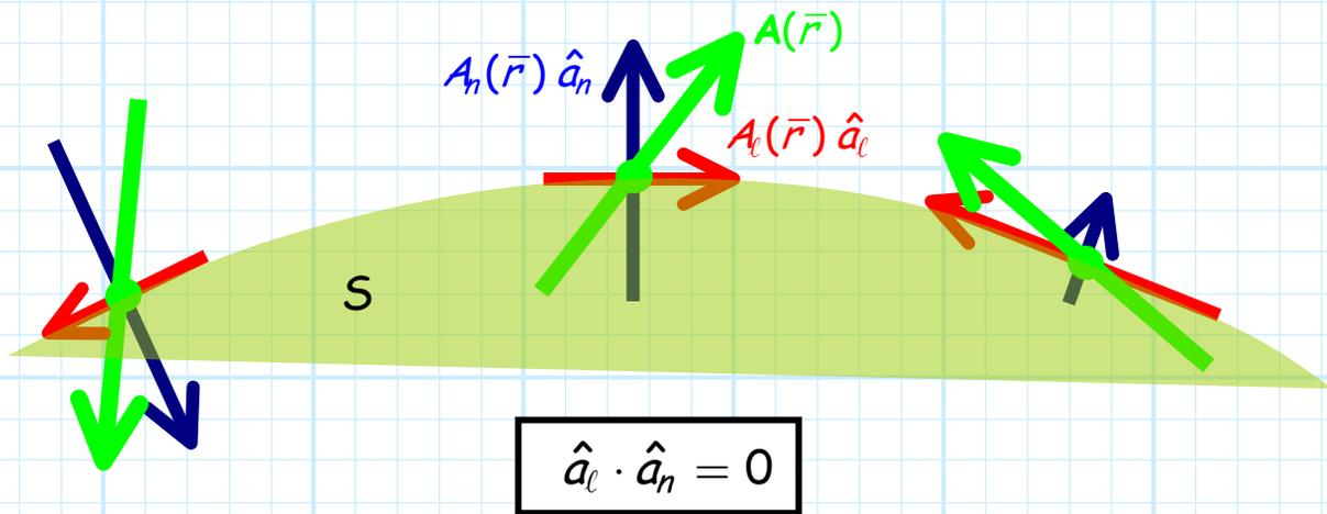
We note that the differential surface vector  $\overline{ds}$  can be written in terms of its magnitude ( $|\overline{ds}|$ ) and direction ( $\hat{a}_n$ ) as:
