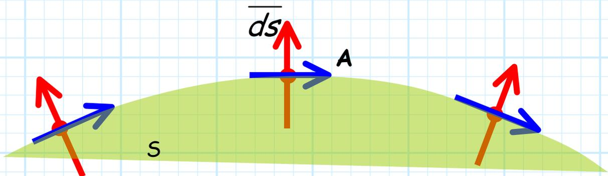
Although  $S$  represents **any** surface, no matter how **complex** or **convoluted**, we will study only **basic** surfaces. In other words,  $\overline{ds}$  will correspond to one of the differential surface vectors from Cartesian, cylindrical, or spherical coordinate systems.
