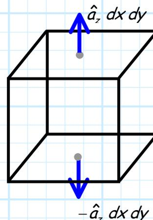
Similarly, we would use differential line vectors of **opposite** directions for each of the pair of side surfaces (left and right), as well as for the front and back surfaces.
