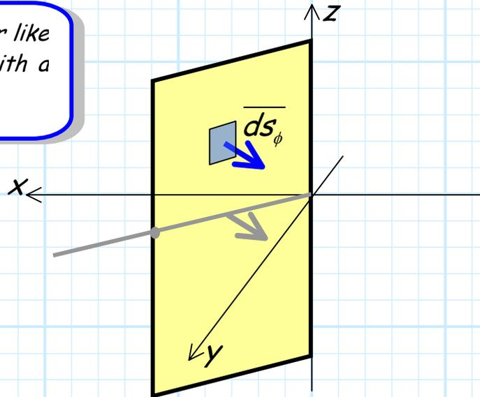
Note the differential surface vector  $\overline{ds}_\phi$  is **orthogonal** to this surface at every point.
