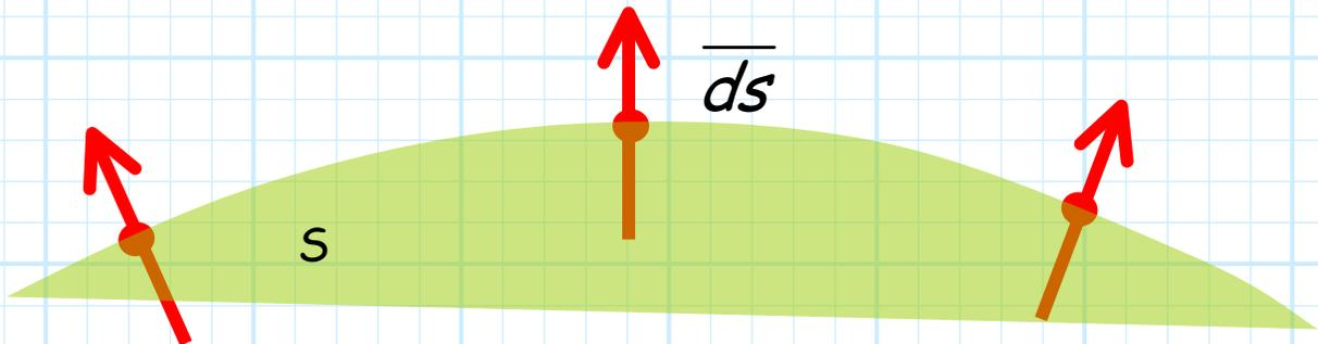
As a result, the differential surface vector  $\overline{ds}$  is **normal** (i.e., orthogonal) to surface  $S$  at every point on  $S$ .
